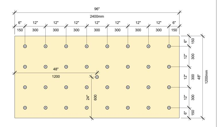
SCHÉMA DE FIXATION POUR ISOLATION: PANNEAU DE 4 PI SUR 8 PI, 33 FIXATIONS
