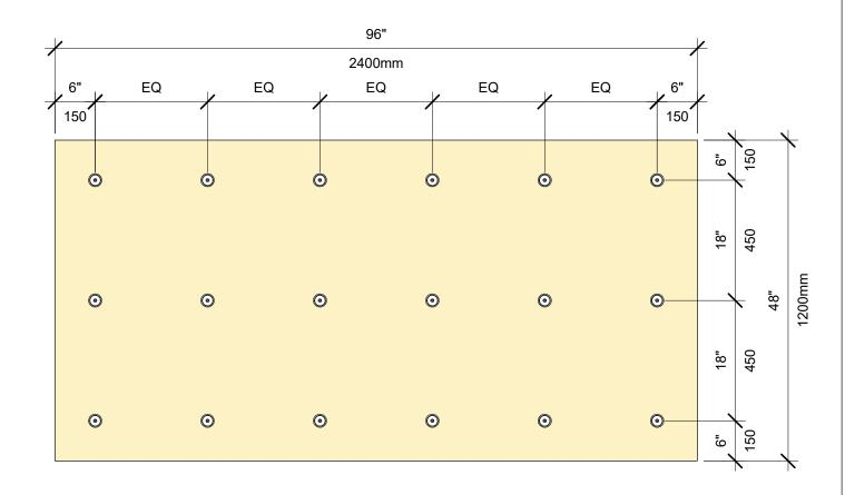
SCHÉMA DE FIXATION POUR ISOLATION: PANNEAU DE 4 PI SUR 8 PI, 18 FIXATIONS
