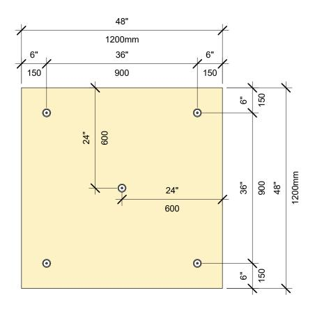
SCHÉMA DE FIXATION POUR ISOLATION: PANNEAU DE 4 PI SUR 4 PI, 4 FIXATIONS
